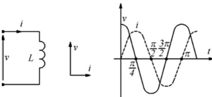
$$\bar{I} = \frac{\bar{V}}{X_L} = \frac{\bar{V}}{jX_L} = \frac{\bar{V}}{j\omega L}$$
