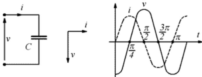
$$\bar{I} = \frac{\bar{V}}{X_C} = -j\omega C \bar{V}$$
